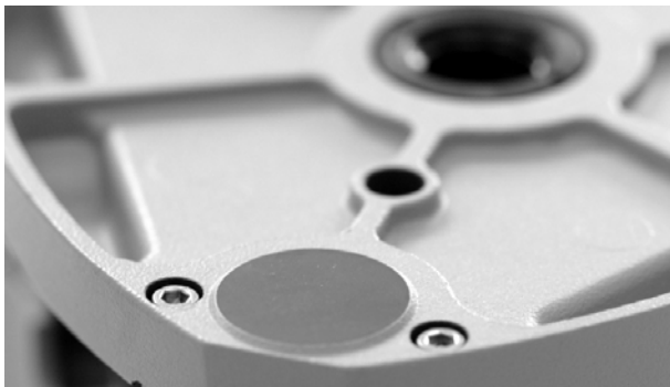
Figure 5 - Bottom side of the base plate of a Leica GDF121 tribrach – shown is one of three supporting areas (points)
