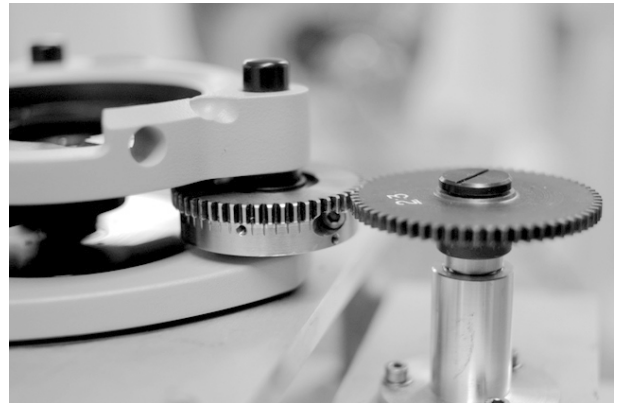
Figure 13 - Tribrach lifetime test setup
