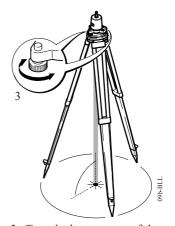
3. Turn the base screws of the tribrach until the laser spot coincides with the ground point.
