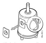
2. Tilt the instrument to allow batteries to slide out
