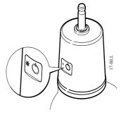
If the diode is flashing the capacity of the battery is too low
