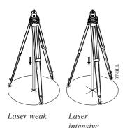
The brightness adjustment remains active even after switching off the basic laser plummet.
