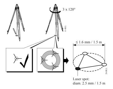
If the centre of the laser spot makes a clearly triangular movement or if the centre of the spot moves away more than 1.4 mm from the first marked point an adjustment may be necessary. Call your nearest Leica Geosystems service workshop.
