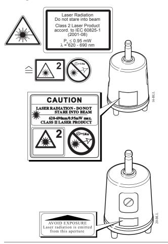
Type: SNLL111 Art. No. 644058 Power: 6V=/200mA max. Leica Geosystems AG CH-9435 Heerbrugg Made in Singapore xxxx Serial No.: xxxxxxxx
