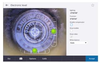
**NOTE** – To see movements in the instrument position reflected as expected in the video plummet display, orient the instrument so the handle is closest to the operator and the instrument is in the Face 1 position. The figures below show how the instrument orientation is reflected in the plummet screen. Moving the plummet forward moves the plummet toward the top of the screen.
