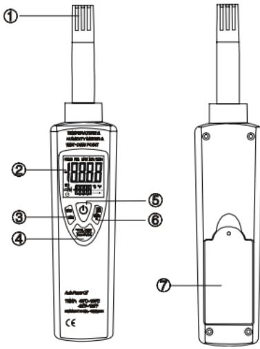
1. Humidity / Air Temperature Probe: Humidity and Temperature Semiconductor Sensor inside.
