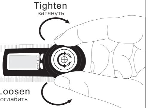
Rotate the ruler to measure the angle.
