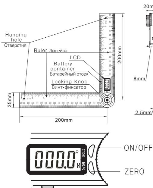
**ON/OFF** Short press ON/OFF to turn on the device. Short press ON/OFF to shut off the LCD. Long press ON/OFF for more than 3 seconds to shut off the whole system. Automatically shut off function in 6 min. Move the scale to turn on the device when at off LCD status.
