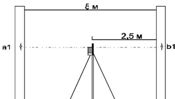
Set up the instrument 0,5-0,7m away from the wall and make, as described above, the same marks. If the difference  $\{a1-b2\}$  and  $\{b1-b2\}$  is less than the value of "accuracy" (see specifications), there is no need in calibration.
