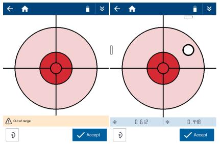
• The electronic bubble will display green with the bubble inside the green target area when the scanner is leveled within compensation range of ±0.5°. The target will turn green once the bubble touches the outer edge of the target but it is important to center the bubble on the green target to ensure the scanner remains within compensation range throughout the full scan. Tap **Accept** when satisfied.
