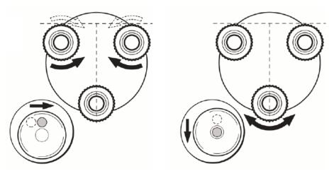
3. Place the scanner on the tribrach and secure it with the tribrach's locking lever.
