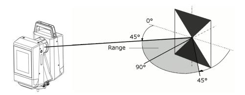
TIP – With a smaller angle of incidence, the possible target distance is reduced. The maximum angle based on the normal of the target should be less than ±45°.
