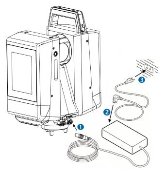
To operate with the power supply:
