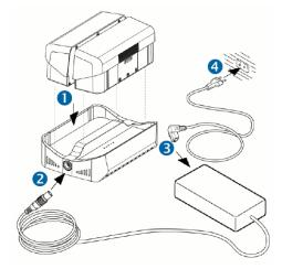
To charge the battery packs with the car charging cable 12 V:
