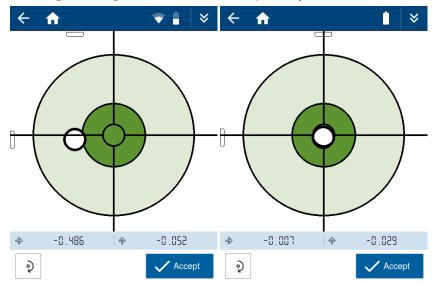
• Tap to execute a level calibration. If you level the scanner perfectly and rotate 180° and it is no longer level then you should perform a level calibration. This may be required after transport or extended storage. The calibration makes two measurements at 0° and 180° to calculate and store the offset.
