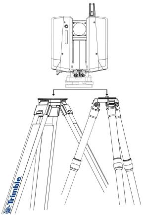
TIP – The scanner can be leveled using the tribrach thumb screws and the integrated electronic level in the onboard UI.
