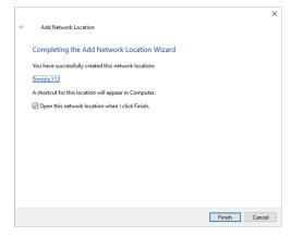
After this action, an explorer window will open showing the project folders that exist on board your X12 scanner. You can now copy or move the required projects onto your PC. 12. After closing this window, the X12 may automatically be added to your Network locations or you may be prompted to add it. The location will be present for future connections when you click on This PC.
