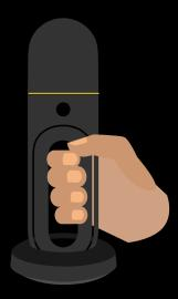
2. While initializing (LED blinking yellow) hold the device stable on the table stand.
